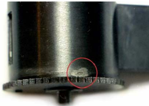
Fig. 7: screw to open the lens turret
