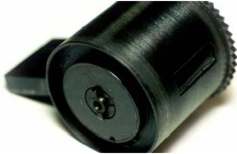
Fig. 6: lens turret viewed from bottom, the spring would sit in the groove
