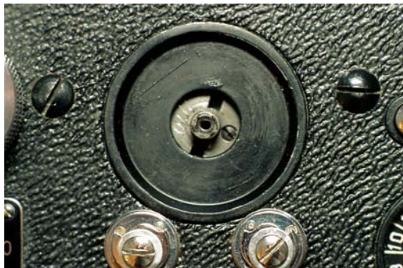
Fig. 2: lens turret viewed through camera top with lever removed
